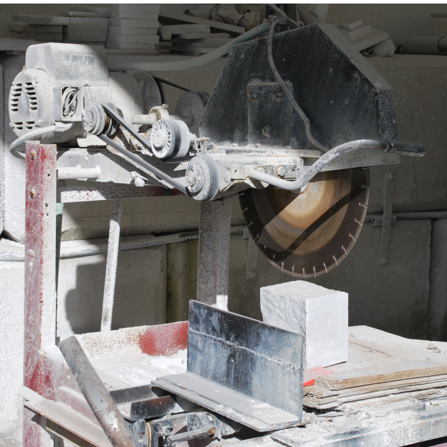
Below/Beside: The small (but huge for most lapidary folks) chop saw and the sliding saw used for the business' smaller projects and finer work. For scale, the block on the chop saw stand was at least a solid eight inches tall.
